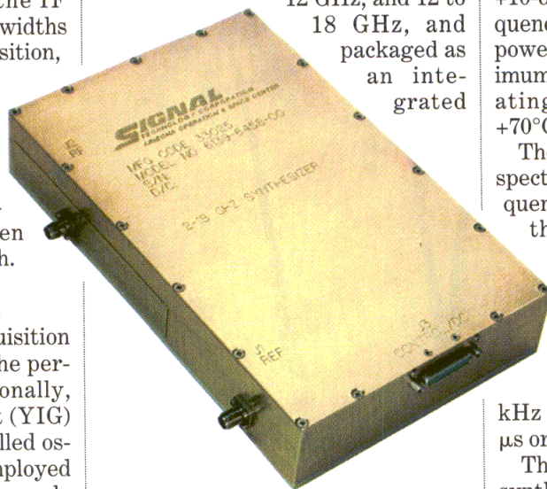
1. Model 6139-6458-00 is a high-performance frequency synthesizer that operates from 2 to 18 GHz in 10-MHz steps with 11-b digital transistor-transistor-logic (TTL) control.
